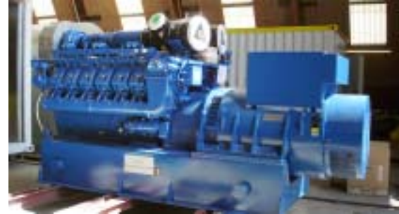
CHP piston engine for assembly in container
